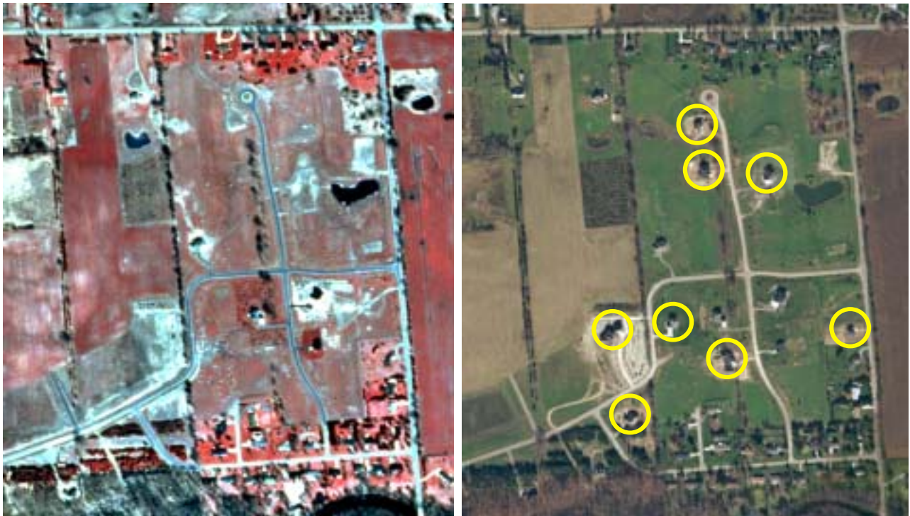
Figure 7. Older, outdated imagery can be a problem in areas experiencing rapid growth. This example shows an area in Williamstown Township, Ingham County Michigan. On the left is a NAPP image from March, 1999 showing an area under development. On the right is a AirphotoUSA image from October 2000 showing the same area with the circles representing new houses constructed since March, 1999.
